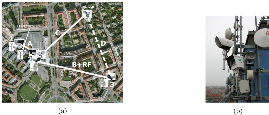
Figure 7: a) deployment of FSO network at the CTU in Prague; b) detail of node 2.
