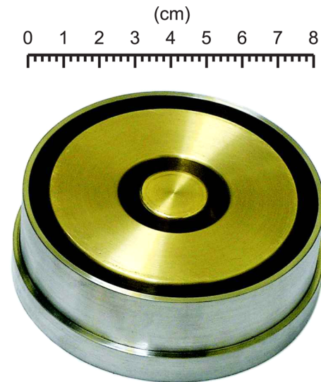
FIG. 1. Nozzle of a double shell gas puff with an inner and outer diameter of 30 and 80 mm, respectively.
