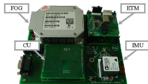
Figure 1. The system for calibration purposes and real-time attitude and heading estimation: (FOG-fibre optic gyro, ETM-electrolytic tilt module, IMU-inertial measurement unit, CU-control unit).
