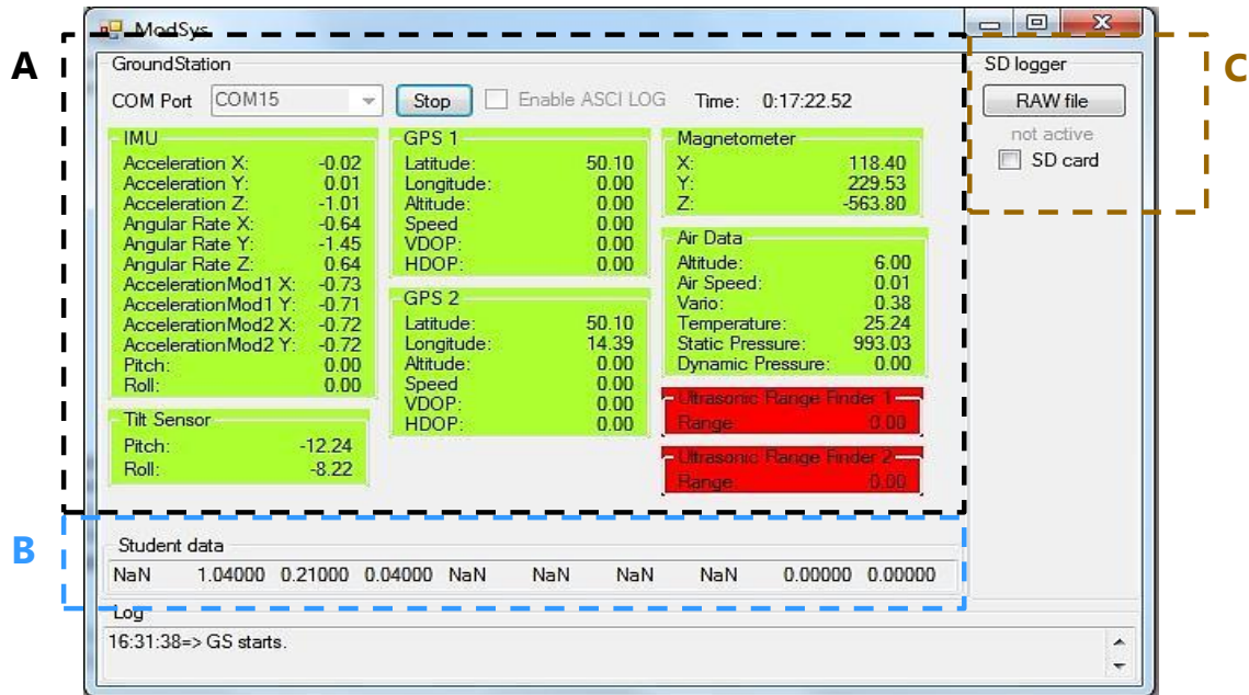
Fig. 17 – The modular navigation SW (ModSys) A – measured and stored data, B – arbitrary data, C – SD logger data proceeding
