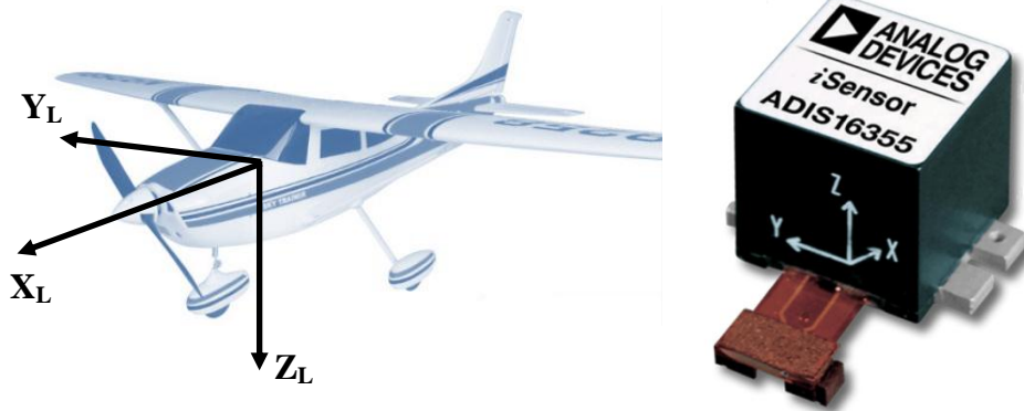
Fig. 5 – Typical framework of the vehicle (left), of the measurement unit (right)
