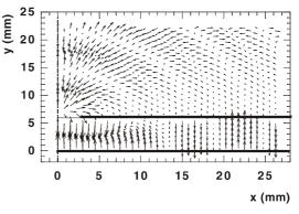
Fig. 6 Computed electric field of the odd space leaky mode corresponding to the 2nd branch of the dispersion characteristic in Fig. 5 on the transversal plane of the ICBSL from Fig. 5 at  $h/\lambda_0=0.35$  (17.5 GHz).
