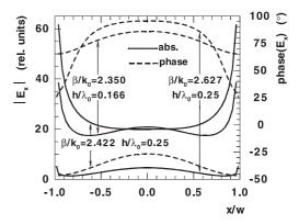
Fig. 11 The calculated distribution of the  $E_x$  field of the 1st leaky mode within the slot of the MICBSL from Fig. 8 at  $h/\lambda_0=0.166$ , the very left point of the ambiguous characteristic, and at its two points when  $h/\lambda_0=0.25$ .
