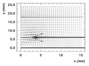
Fig. 9 Computed electric field of the even dominant bound mode on the MICBSL from Fig. 8 at the normalized frequency  $h/\lambda_0=0.04$ .
