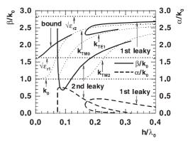
Fig. 10 Dispersion characteristics of even modes on the MICBSL with w=6 mm,  $h_1$ =6 mm,  $h_2$ =9 mm,  $\epsilon_{r1}$ =2.6,  $\epsilon_{r2}$ =7 and  $\epsilon_{r3}$ =1.
