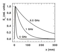
Fig. 4 Computed distribution of the  $E_y$  field in the substrate perpendicular to the line axis, at the level y=3 mm for the ICBSL from Fig. 2 at three frequencies. The fields are normalized to 1.
