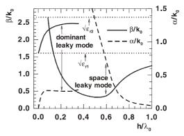
Fig. 2 Dispersion characteristics of even modes on the ICBSL with w=6 mm, h=6 mm,  $\epsilon_{r2}$ =7 and  $\epsilon_{r1}$ =2.6.
