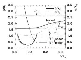
Fig. 13 Dispersion characteristics of the odd space modes on the MICBSL with w=12 mm,  $h_1=6$  mm,  $h_2=3$  mm,  $\epsilon_{r1}=2.6$ ,  $\epsilon_{r2}=7$  and  $\epsilon_{r3}=1$ .
