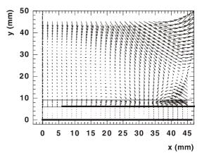
Fig. 14 Computed electric field of the odd space leaky mode corresponding to the characteristic "1" from Fig. 13 at  $h/\lambda_0=0.14$  (7 GHz).
