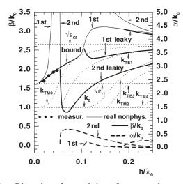
Fig. 8 Dispersion characteristics of even modes on the MICBSL with w=6 mm,  $h_1$ =6 mm,  $h_2$ =12 mm,  $\epsilon_{r1}$ =2.6,  $\epsilon_{r2}$ =7 and  $\epsilon_{r3}$ =1.
