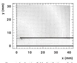
Fig. 3 Computed electric field distribution of the even dominant leaky mode on the transversal plane of the ICBSL from Fig. 2 at  $h/\lambda_0=0.1$  (5 GHz).
