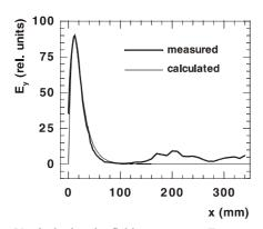
Fig. 12 Vertical electric field component  $E_y$  measured and calculated on the top surface of the glass slab of the MICBSL from Fig. 8 at  $h/\lambda_0$ =0.04 (2 GHz).
