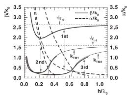
Fig. 5 Dispersion characteristics of odd space leaky modes on the ICBSL with w=6 mm, h=6 mm,  $\epsilon_{r2}$ =7 and  $\epsilon_{r1}$ =2.6.
