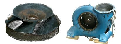
FIGURE 2. Cloud point of the runner (left) and the volute of the turbine (right).
