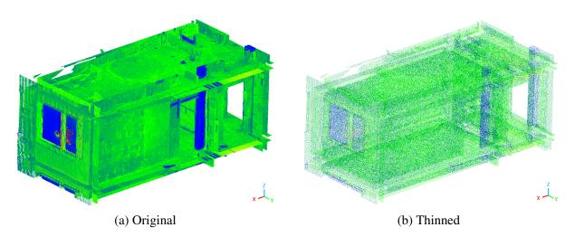
Figure 4.2: Comparison of point cloud data before and after density thinning with CloudCompare.
