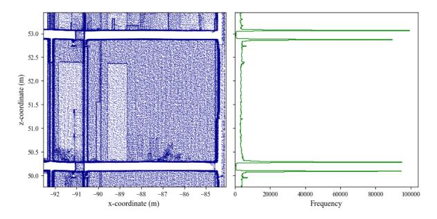
Figure 4.3: Point cloud cross-section (on the left). A z-coordinate histogram of point cloud data to detect slab surface candidates (on the right).
