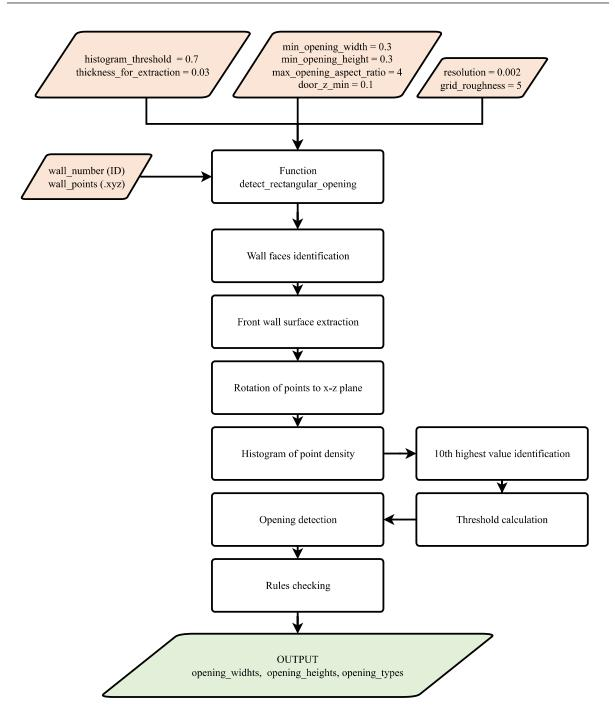
Figure 4.13: A flowchart describing algorithm for openings detection.
