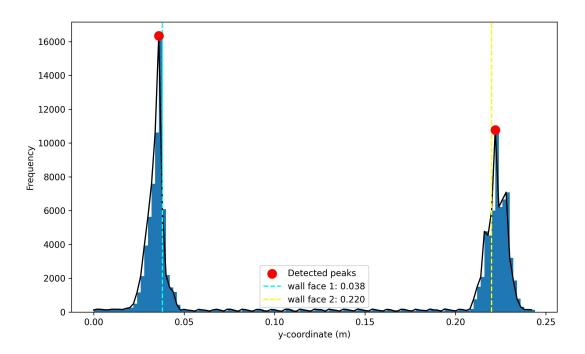
Figure 4.11: The histogram of the density of points on the y-coordinate along with vertices identified and vertical lines indicating the positions of the wall surfaces.
