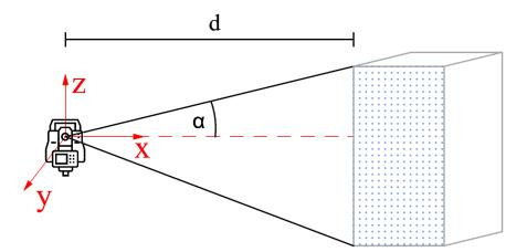
Figure 3.1: Principle of Laser Scanning. " $\alpha$ " represents the elevation angle, and "d" denotes the horizontal distance.
