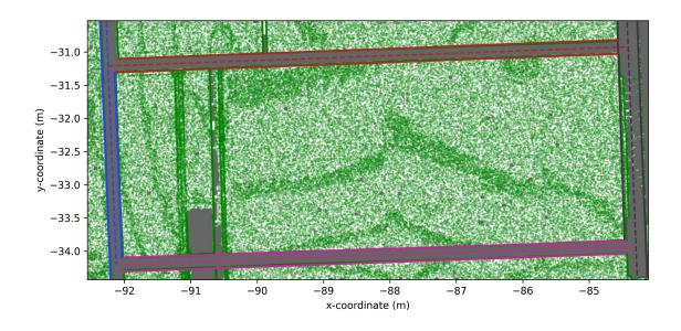
Figure 4.5: Final walls (colored) segmented from point cloud (green). On the background mask.
