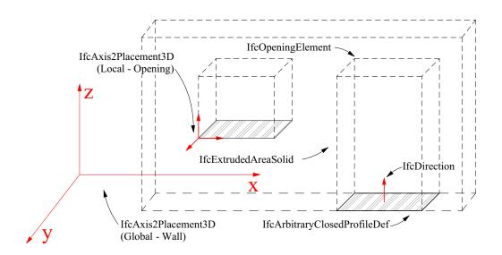
Figure 4.18: Main IFC classes used to create geometric representation of opening.
