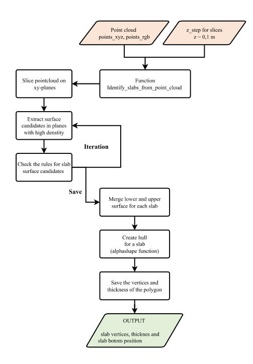
Figure 4.9: A flowchart describing the code for the algorithm for detecting slabs.
