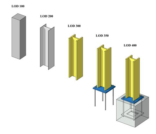
Figure 2.1: Level of Development of steel profile column. Author's own illustration based on [34].
