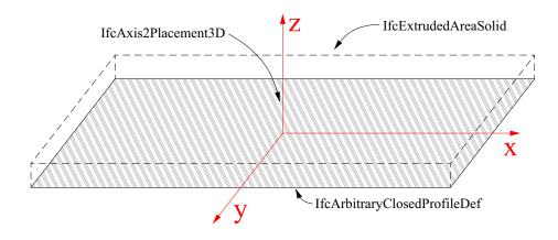
Figure 4.16: Geometric representation of slab created by ifc sweptsolid geometry.
