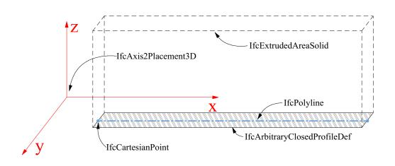
Figure 4.17: Main IFC classes used to create geometric representation of wall.
