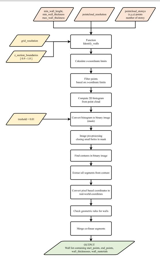
Figure 4.12: A flowchart describing algorithm for walls detection.
