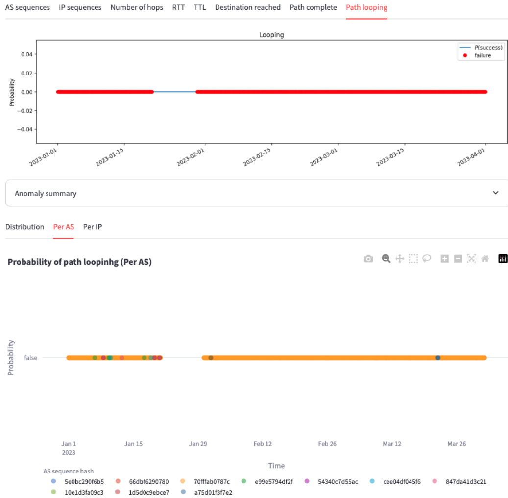
■ Figure C.11 Screenshot of dashboard section related to looping of traceroutes
