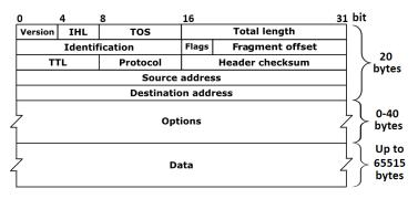
Figure 1.1: Structure of the IPv4 packet. Source: [3]
