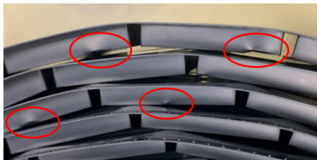
Figure 2.12: Deformation of packaging compartments (circled in red) visible from the side of the reel.
