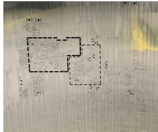
Figure 1.8: Stencil used for the bottom side of the BSRF EA PCB
