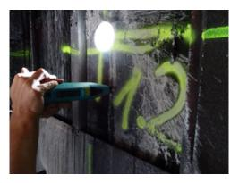
FIGURE 10. Rebound hammer test.
