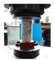
FIGURE 11. Concrete core destructive compressive strength test.
