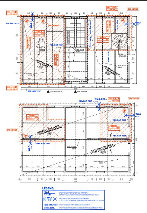
FIGURE 7. Layouts of the first floor (top) and the second floor (middle) with the information regarding the structural diagnostics; legend of the symbols used in the layouts (bottom).
