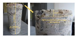
FIGURE 12. Concrete sample from ZONE 1 (WA.2) – estimation of approximate damage depth using colorimetry method.
