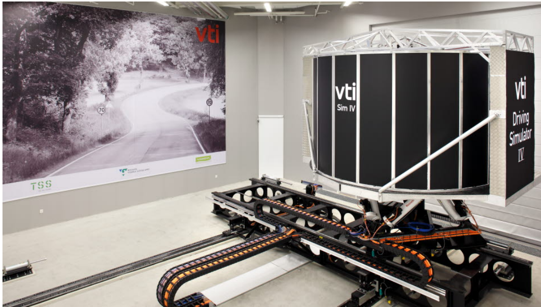
Figure 2.9: A full-size driving simulator (Hejdlösa bilder, 2023)
