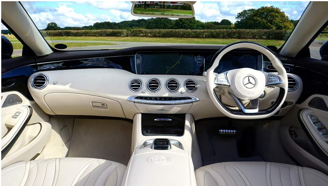
Figure 2.4: Infotainment screen of Mercedes convertible with a supplementary set of controls in the base of the central console
