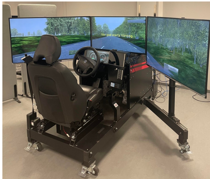
Figure 2.8: An example of a light driving simulator (Ondomiši, 2023)
