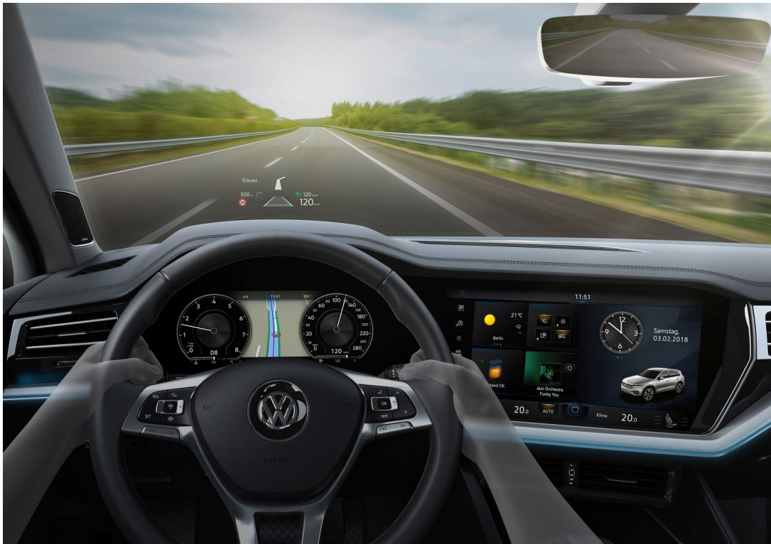
Figure 2.5: Cockpit view of Volkswagen Touareg with a Head-up Display (Volkswagen, 2018)
