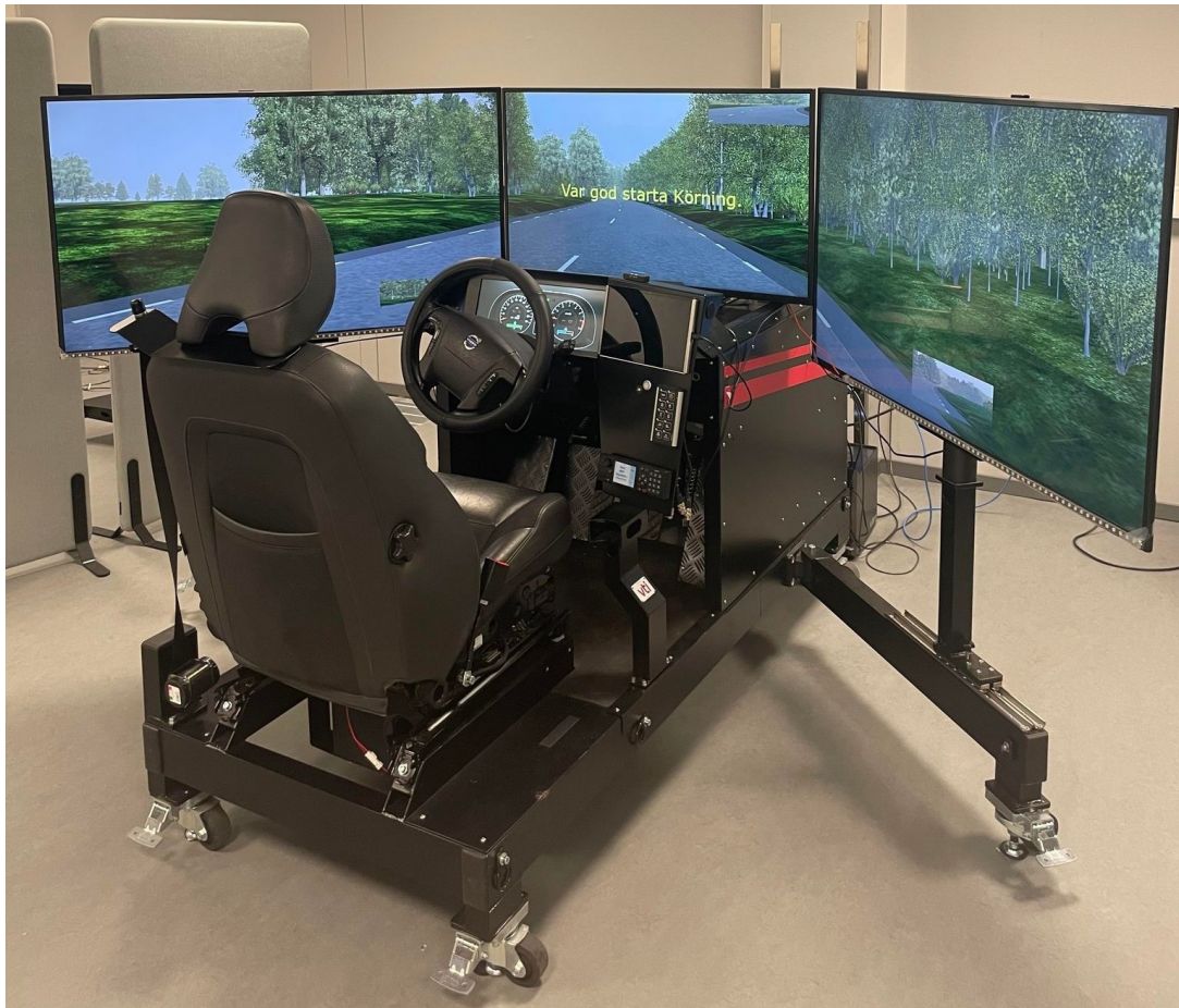
Figure 3.1: Simulator setup (Ondomiši, 2023)
