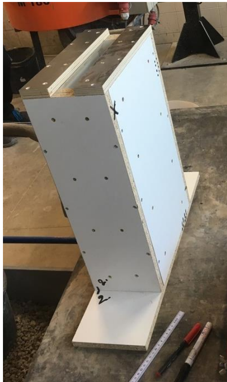
Figure 10 Mould constructed in UCEEB, CTU Prague as preparation for concrete blocks from PPG 100% mixture.
