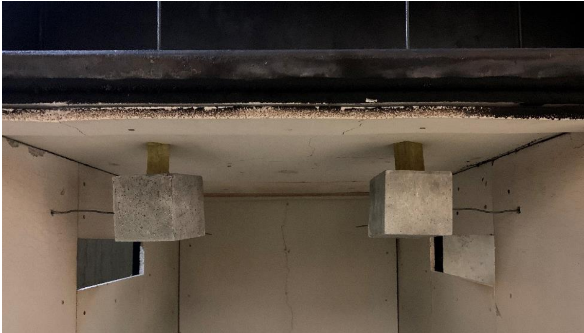
FIGURE 1. Test specimens before the fire resistance experiment.
