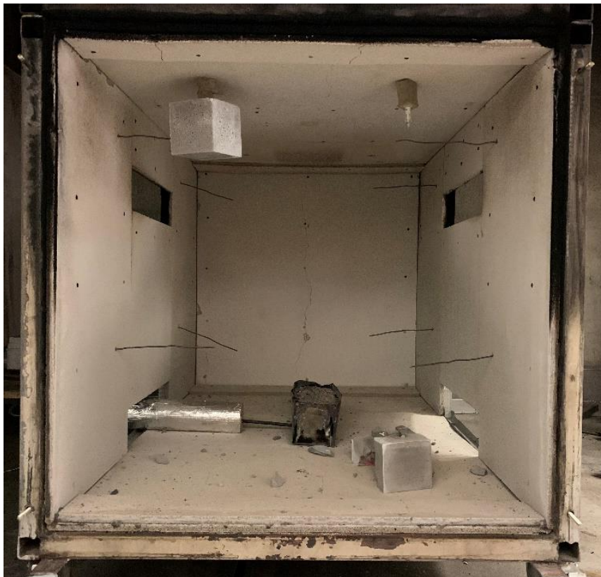
FIGURE 4. Tested samples after the fire resistance experiment.
