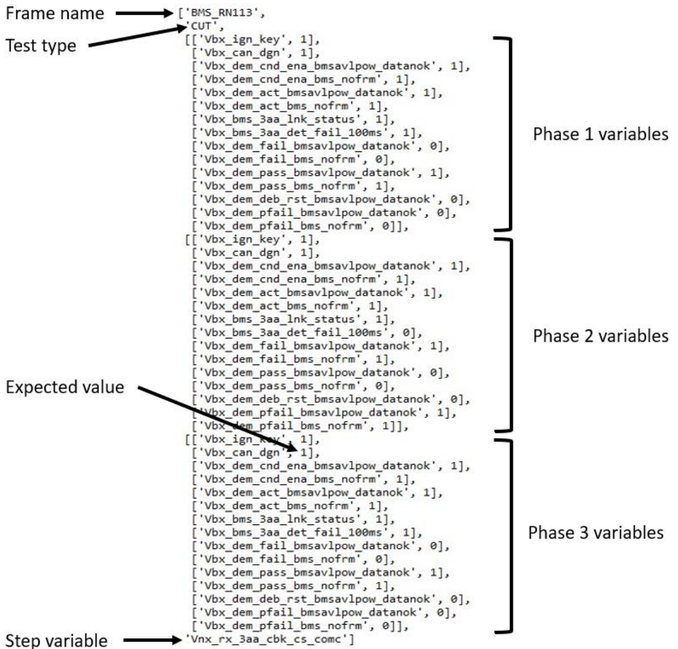
Figure 15 Extracted PVAL HIL of a CUT test in Python
