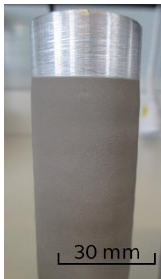
Fig. 5 - Aluminum tube substrate with cold sprayed NiTi coating.
