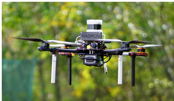
Figure 1.1: A UAV built on quadcopter Tarot T650 airframe [6] with a 3D LiDAR used for the experiments in this thesis.
