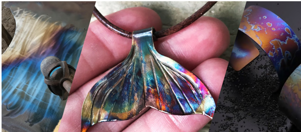
Figure 5.93: Examples of heat coloring on metals: steel by Jeffrey H Dean [39], copper by Mari [40], titanium by Robert Lopez [41].
