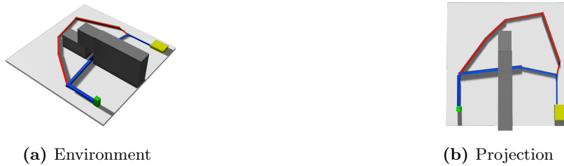
Figure 3.6: The blue path from the start (green) to the goal (yellow), which uses a narrow passage that disappears with top-down projection. The blue path would be impossible to find in the projection. Instead, the red path which is not optimal would have to be used. If the obstacle was even longer, it would be impossible to find a path in the projection
