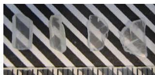
Fig. 2. Prepared samples for optical measurements in order from left to right: CHC-0%, CHC-0.1%, CHC-0.5%, CHC-1%.
