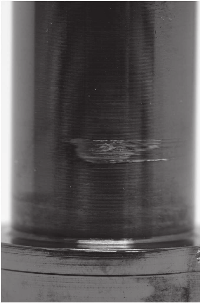
Fig. 6. Pivot damage of the coated implant.
