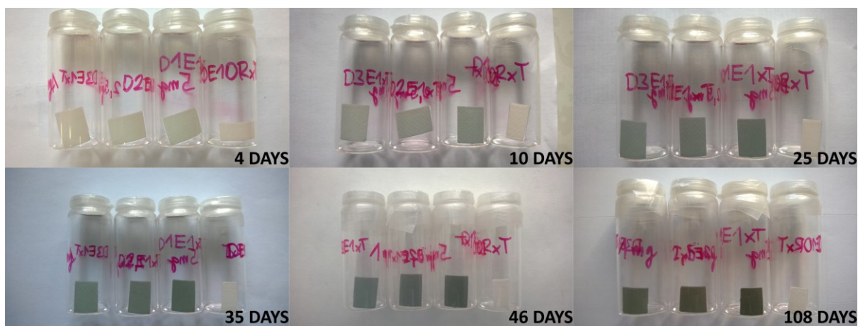
Fig. 9 The genipin cross-linking reaction in collagen samples kept in 100% ethanol with three different genipin to collagen weight concentrations (from left in each photograph: 1:1, 2.5:1 and 5:1) at room temperature for up to 108 days. The sample container on right in each photograph contains a collagen sample immersed in 100% ethanol without genipin (control sample).
