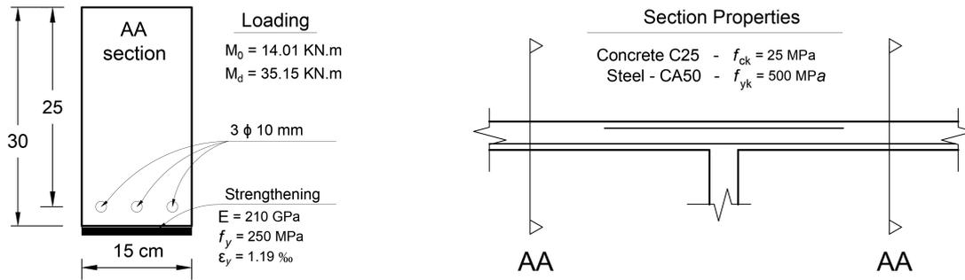
FIGURE 4. Representation of beam characteristics of the building.
