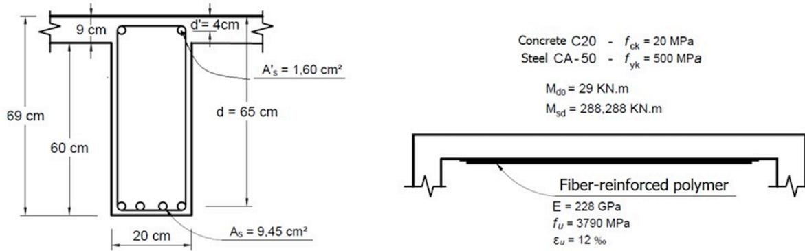
FIGURE 3. Strengthened beam scheme. Source: Adapted from Machado [2].
