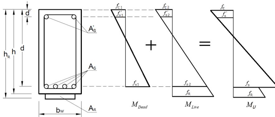
FIGURE 1. Stress diagram of a strengthened beam. Source: Adapted from Silveira [6].
