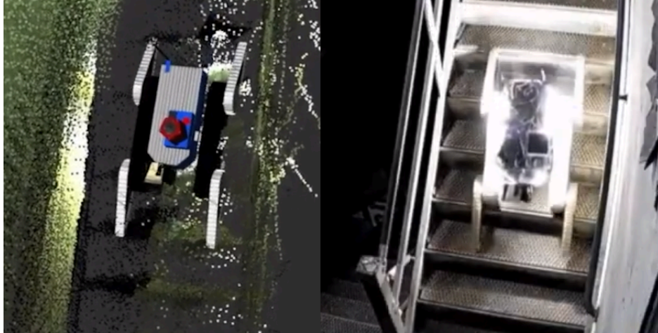
Figure 3.11: Autonomous flipper control in the DARPA subterranean challenge Urban circuit. The robot was remotely given waypoint goals on the map. The path follower algorithm controls the robot velocity, and our flipper controller sets the flippers in such a position that enables a smooth transition.
