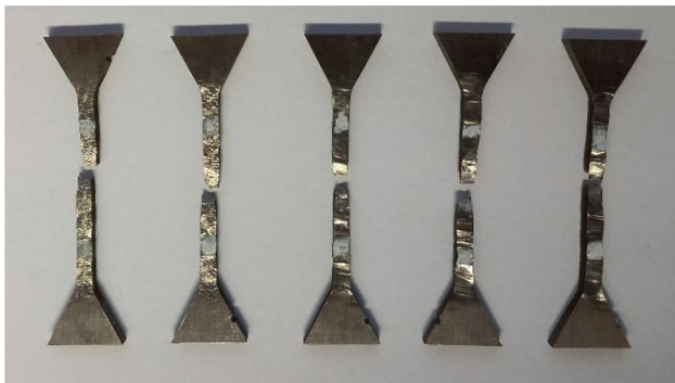
Fig. 21 Tensile testing: example photography of ruptured specimen (CMT discontinuous WAAM—vertical—20 °C)
