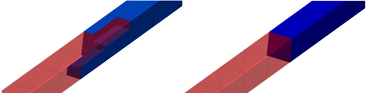
Figure 3: Interfaces between subdomains provided by a graph partitioner (left) and by a geometric partitioner (right).
