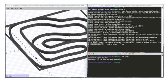
Figure 5.2. Running the Follow the Gap application in the Stage simulator in ROS 2 on macOS 10.14.6  $\,$
