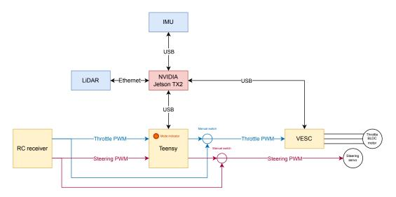
Figure 4.3. Overview of main components with depicted methods of communication. The yellow blocks are part of the low-level system, which always works independently of the main high-level system (NVIDIA Jetson TX2).
