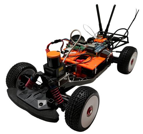
Figure 4.1. The CTU's tx2-auto-usa F1/10 Model Car based on NVIDIA Jetson TX2.
