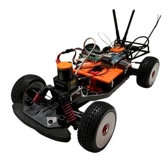
Figure 1.1. One of the CTU's F1/10 Autonomous Model Cars.
