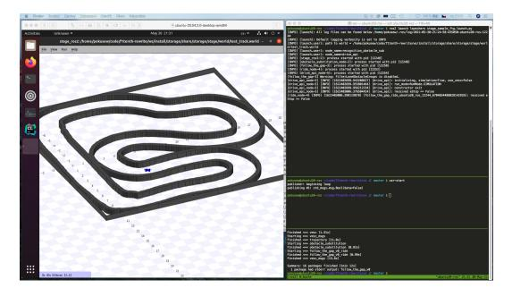
Figure 5.1. Running the Follow the Gap application in the Stage simulator in ROS 2 on Ubuntu 20.04 (as a VM on macOS)
