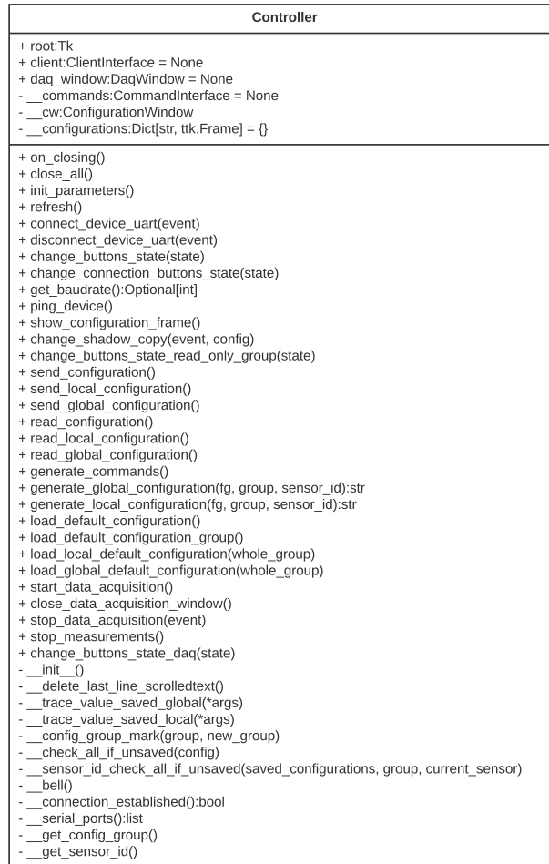
Figure 10: Class diagram of Controller.
