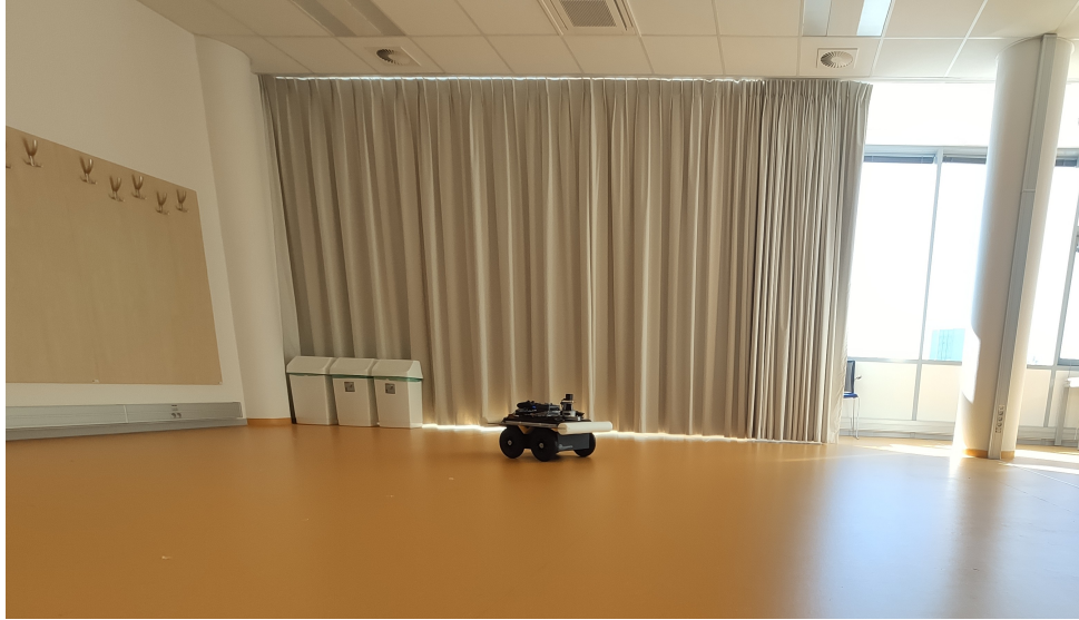
Figure 5.14: Robot Jackal in the room B670. In the back, there is a curtain, which caused a deterioration in the accuracy of the NDT method in the final experiment because of its movement caused by a wind.
