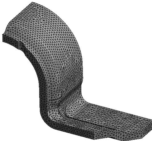
Figure 6.3: Refined mesh with quadratic tetrahedral elements.
