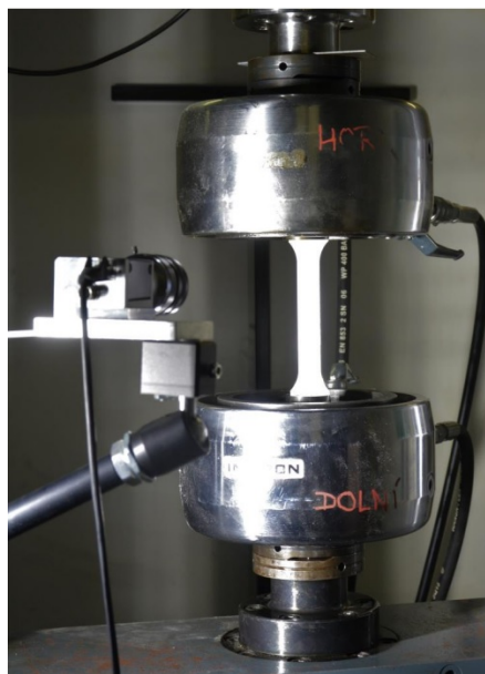
Figure 4.2: Tensile testing rig.[Comtes] Figure 4.3: Geometry of the specimen. [Comtes]
