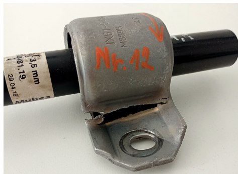
Figure 5.11: Clamp fracture due to fatigue.
