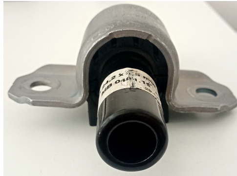
Figure 5.2: Clamp with rubber bearing (testing assembly for fatigue life evaluation).
