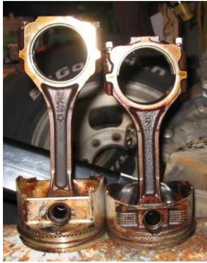
Fig. 53 Comparison of connecting rod length and piston height (57)
