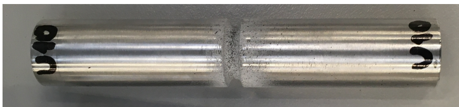
Figure 5.3: Specimen with U-notched sprayed with two acryl paints for DIC measurement.
