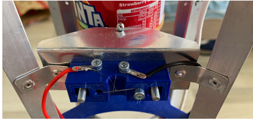
Fig. 3.27: Final nylon attachment part shown in use on the release system prepared before ejection test
