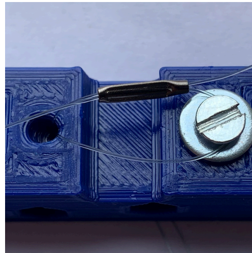
(b) Brass tube used to crimp two ends of a nylon line
