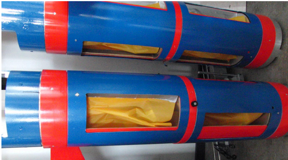
Fig. 2.9: NAVRO CanSat release system [10]
