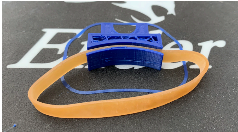
(a) Picture taken while the printing process was paused to allow for rubber band insertion
