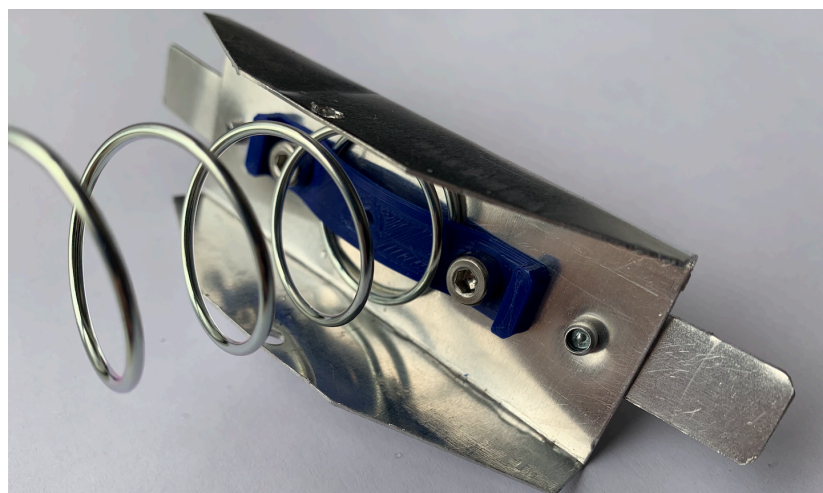
Fig. 3.28: 3D printed spring retainer shown in blue with oval holes to adjust springs position relative to the center hole
