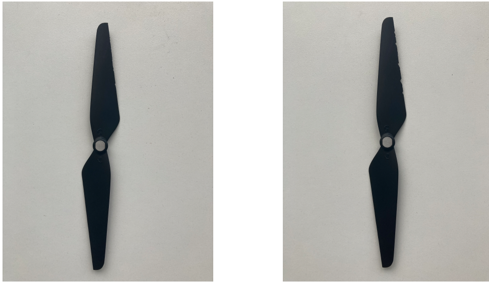
(a) Small mechanical damage
