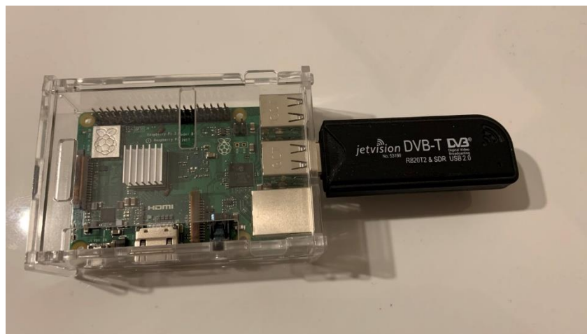
Figure 7 – ADS-B receiver without connected antenna
