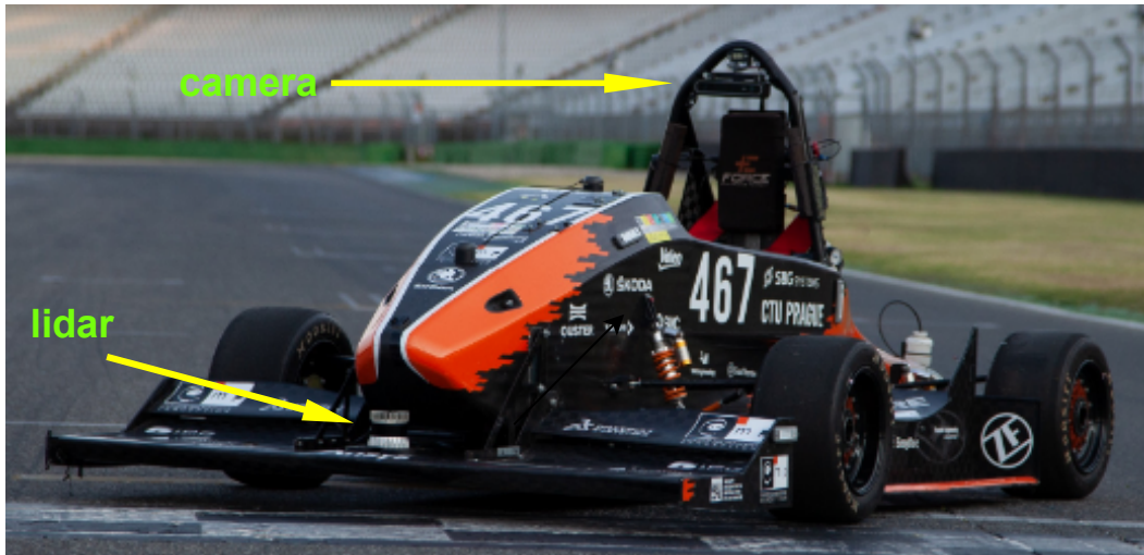
Figure 5: Photo of the FEE eForce Driverless autonomous formula. The lidar is positioned on the front wing and the camera is mounted on the main hoop of the car.
