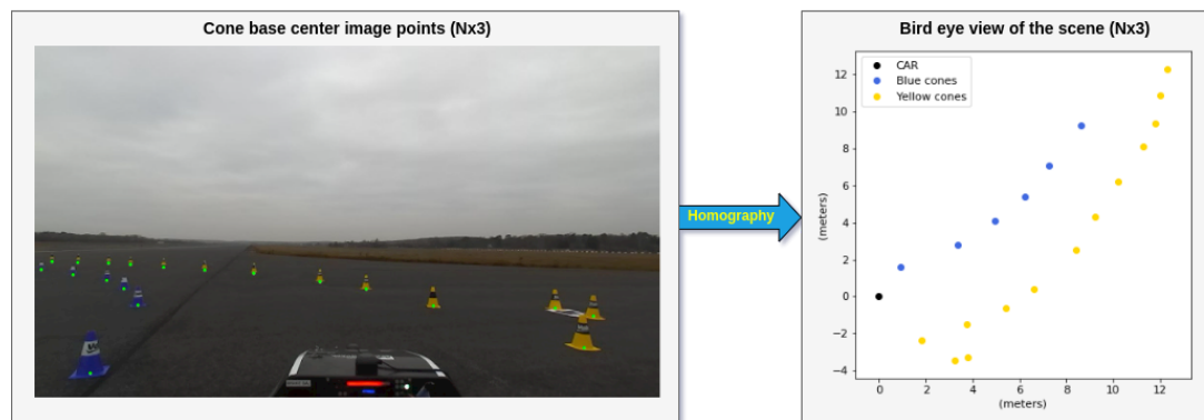
Figure 13: The process of projecting cone base center image points into the car coordinates with a homography matrix, creating a local map of the scene.
