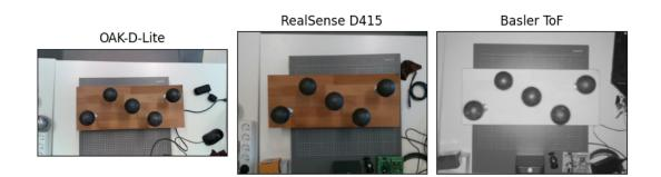
**Figure 4.1** Wrought iron spheres shot from the distance of 700 mm.
