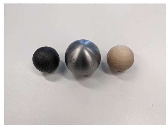
**Figure 3.2** Wrought iron sphere, aluminium sphere, and wooden sphere with a radius of 30 mm, 40 mm, and 30 mm, respectively
