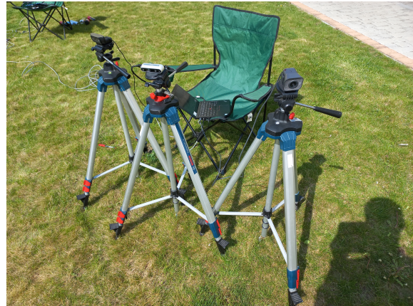
(b) Cameras for recording. Left to right: Logitech C920, Intel RS D435, Logitech C980
