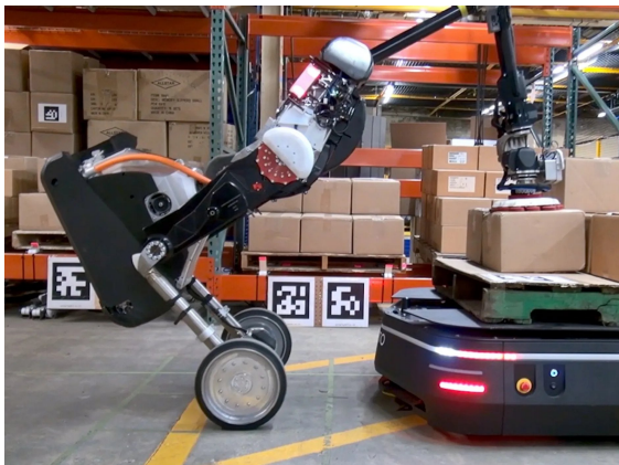
Figure 11: AprilTag markers as labels for warehouse robot [49]
