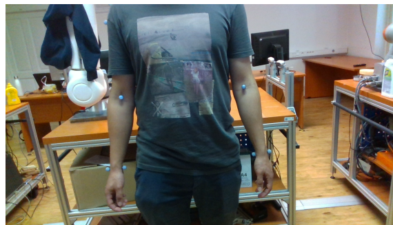
Figure 4.18: Image of the participant in the absolute evaluation of 3D human pose experiment with visible reflective markers placed on the body keypoints.
