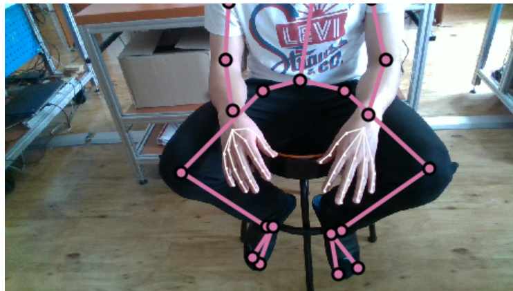
Figure 4.15: Example image during experiment with detected human body keypoints and RealSense position adjusted with tilt.
