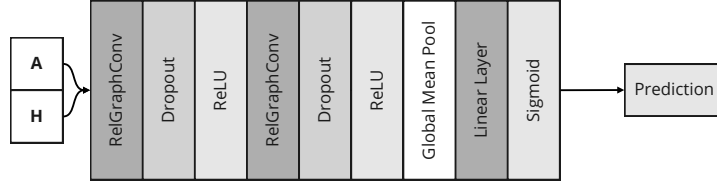
Figure 6.1: The graph neural network uses adjacency matrix A and initial node feature vectors for every node H . Our architecture is two Relation graph convolution layers with ReLU activation function and dropout. Next, we perform global mean pooling over node embeddings, resulting in single vector for entire graph. This vector is then processed using Linear layer and Sigmoid activation function.
