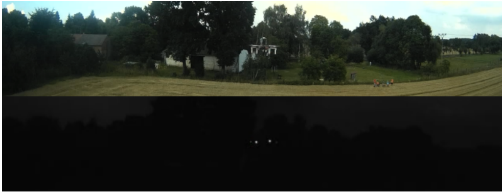
Figure 3.1. Comparison between visible and UV camera footage from UVDAR. The UV image is significantly easier to process to retrieve UAV information [2].
