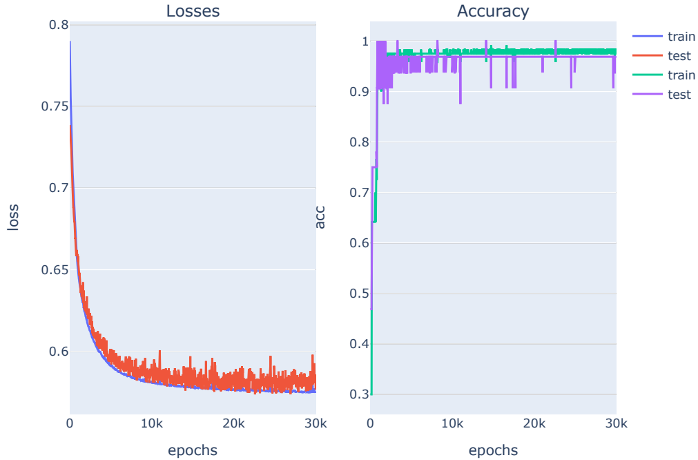
Figure 3.15: Values of the binary cross-entropy loss function and the classification accuracy on the train and the test sets.
