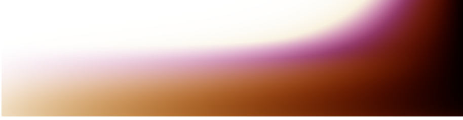
Figure 5.11: The transmittance texture characterizing the optical depth of the atmosphere.
