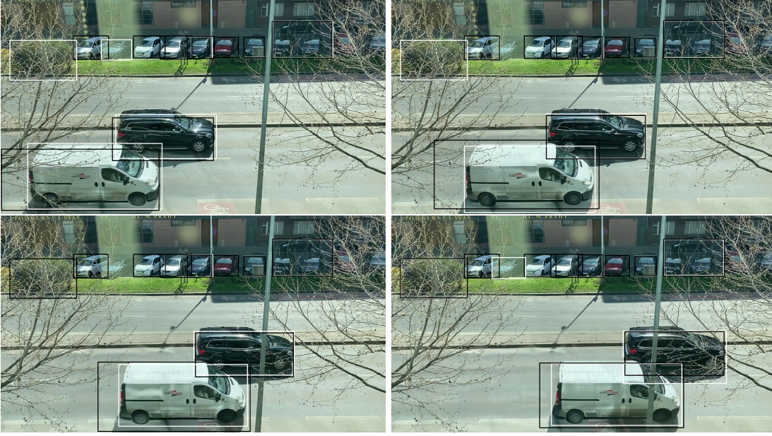
■ Figure 5.2 Tracking on 4 sequential frames. Detected vehicles are bordered with white while tracking predictions are black. We can notice a couple of false detections at the top (a bush). Since they are not located on the road they do not cause problems to the vehicle counting.
