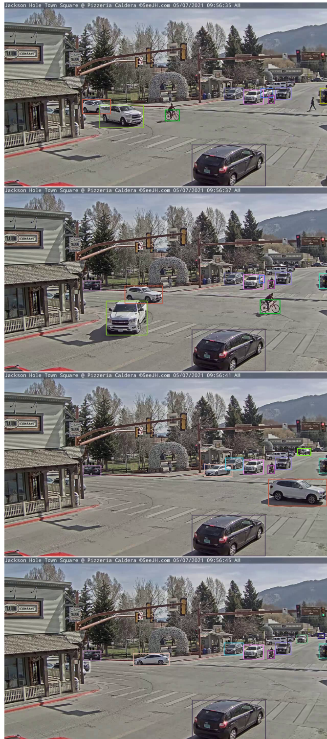
■ Figure 2.8 An example of multiple vehicles movement tracking. The same vehicle is bordered with the same color.
