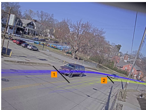
■ Table 7.7 A side view of an in-town road. The position of the camera is fine as it provides a clear view of both tracks without notable overlaps of vehicles. This results in an average 1.0 accuracy (experiment #3).
