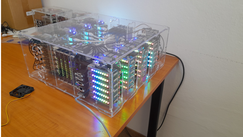
Figure 8.1: Pico 48 cluster running Blinker task
