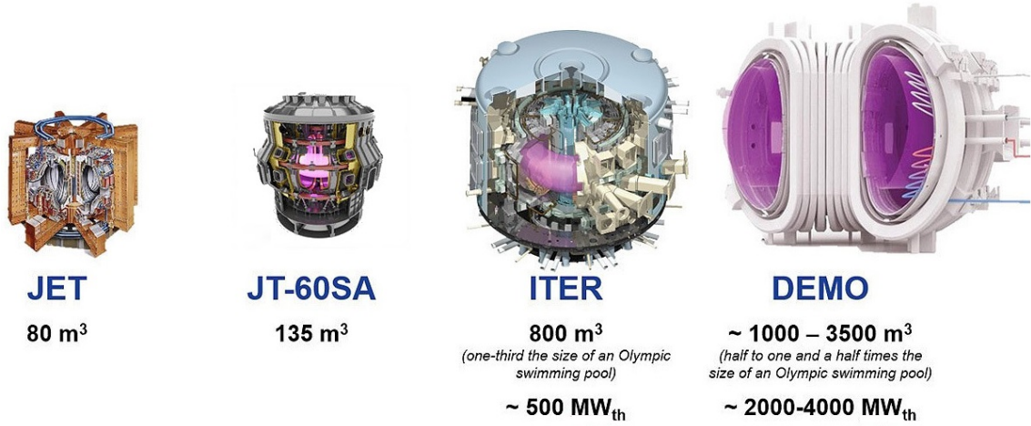
Figure 8: Planned development of tokamaks with the aim of achieving economically acceptable fusion energy. It is worth mentioning the just being launched Japanese tokamak JT-60SA, which should replace the function of the old JET tokamak by following a complementary research and development programme of future fusion power plants. Obtained and modified from [26].
