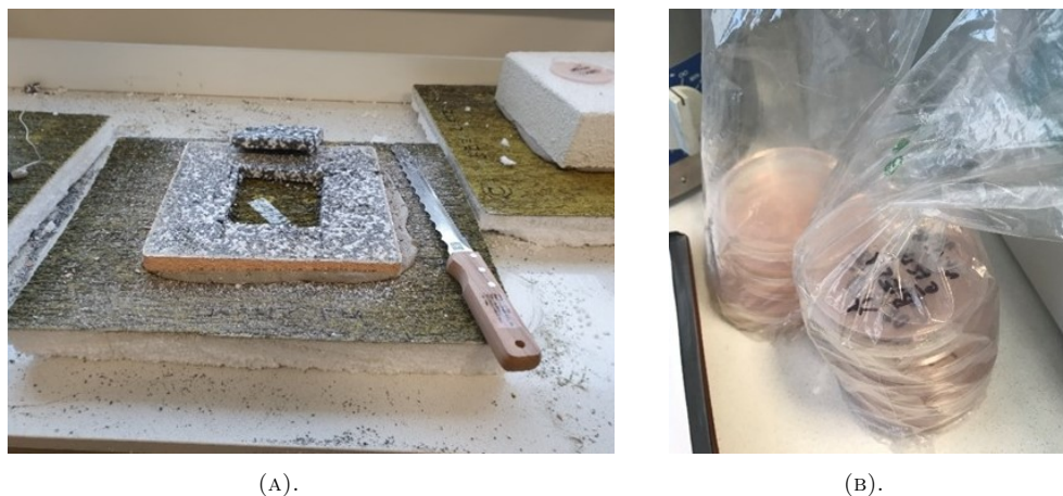
FIGURE 7. Removal of second layer of insulation. Sampling of biological material with sampling tape into petri dishes immediately after the opening of the gap.
