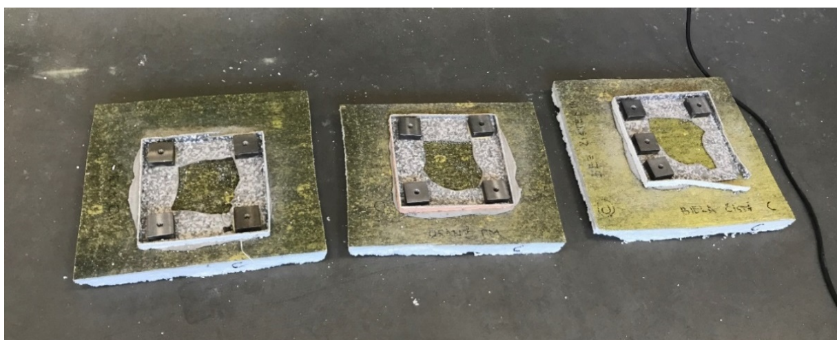
FIGURE 10. Removal of second layer of insulation. Preparation of samples in each group to test adhesiveness on the sample: from the right, C, B, A.
