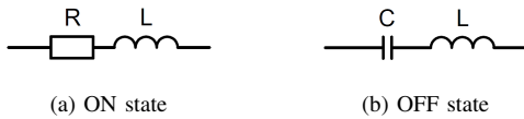
Fig. 17: RLC equivalent circuits of PIN diode used in the simulations for ON and OFF state.
