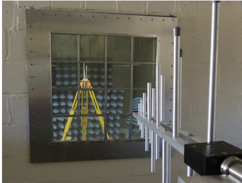
Figure 16: Measurement - optically transparent FSS design.
