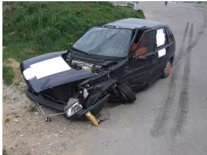
Fig. 17: Small vehicle deformation after road barrier crash test
