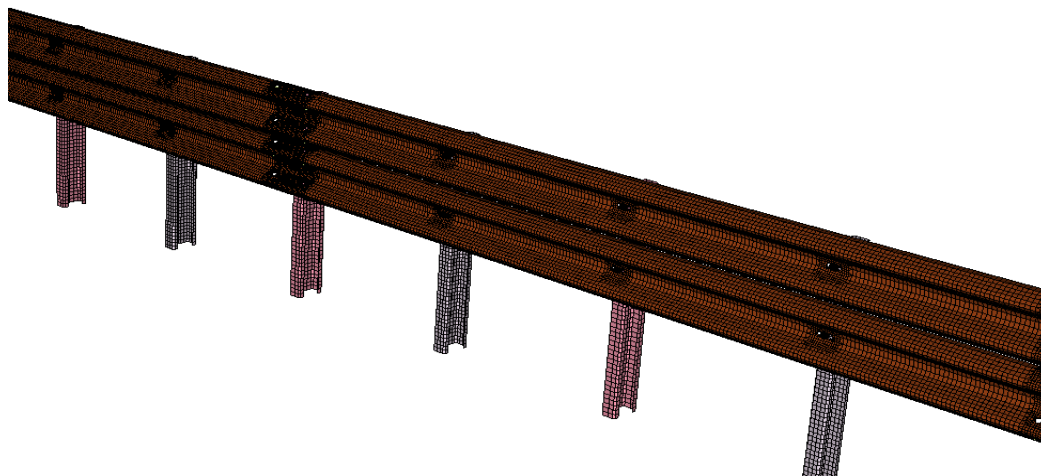
Fig. 39: Road barrier FE model
