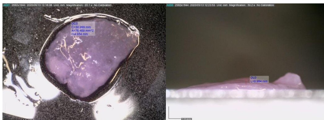
Figure 5.9 Molded cylinder shape, 2 mm height
