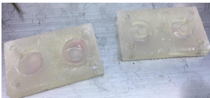
Figure 5.2 Unsuccessful test for 2 mm height due to surface tension
