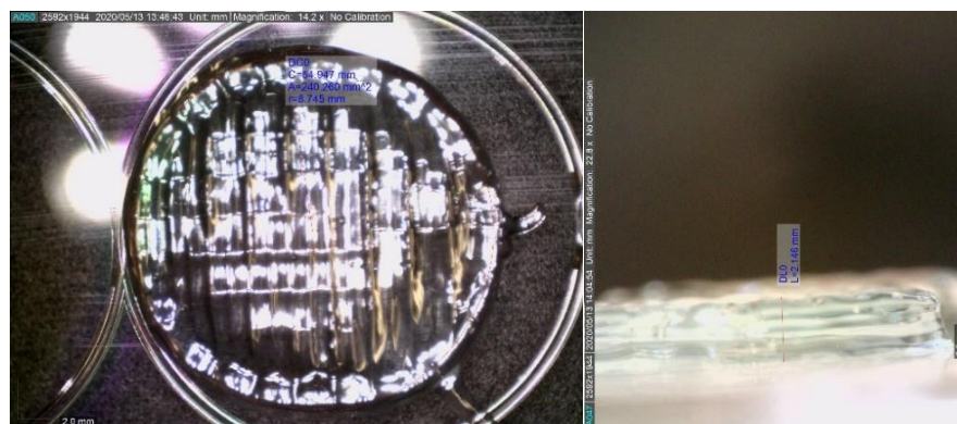
Figure 5.16 Cylinder shape bioprinted at 25 kPa
