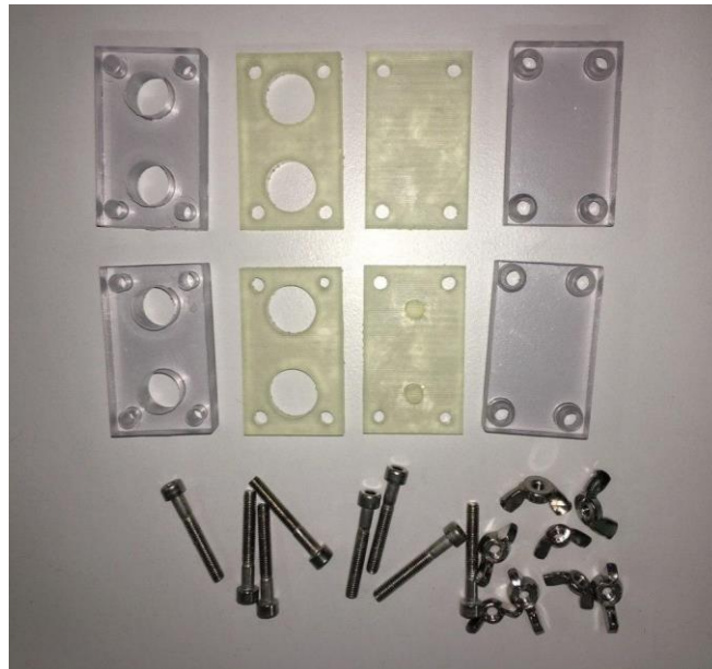
Figure 4.4 3D printed mold forms with nuts and screws, disassembled
