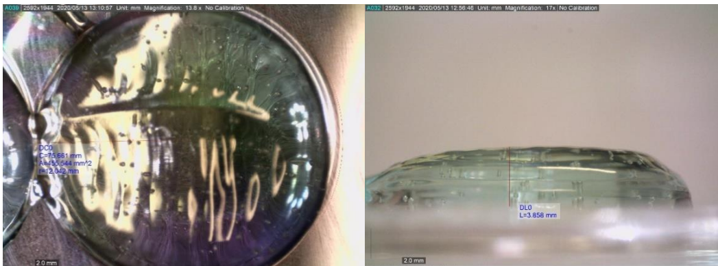
Figure 5.12 Cylinder shape bioprinted at 35 kPa
