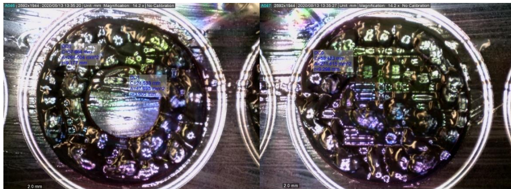
Figure 5.17 Toroid and cylinder shapes bioprinted at 15 kPa
