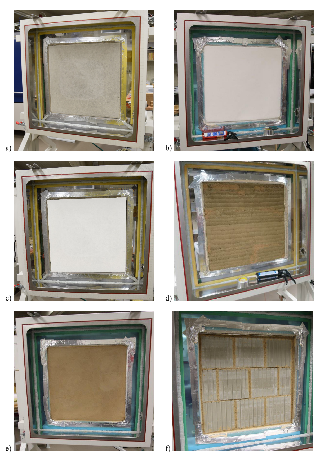
Fig. 62 Testing structures in the climatic chamber: a) concrete wall; b) ceramic hollow blocks with lime plaster; c) partition wall from gypsum board; d) rammed earth panel (C_S10/W10); e) unburned clay hollow blocks with clay plaster; f) fair-face brickwork from unburned clay hollow blocks
