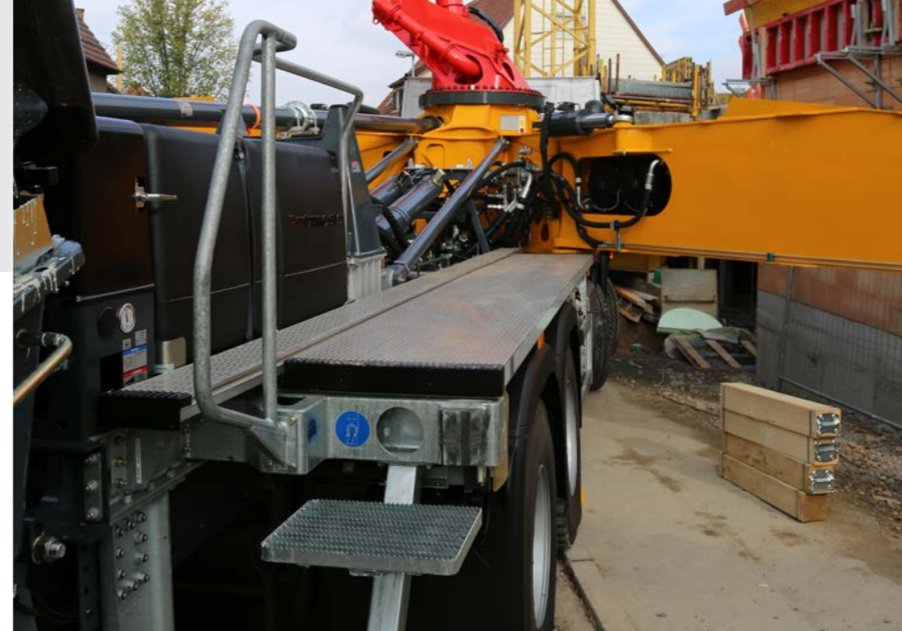
The wide flatbed with anti-slip surface offers a great deal of freedom of movement when working as well as simultaneously providing storage space.
